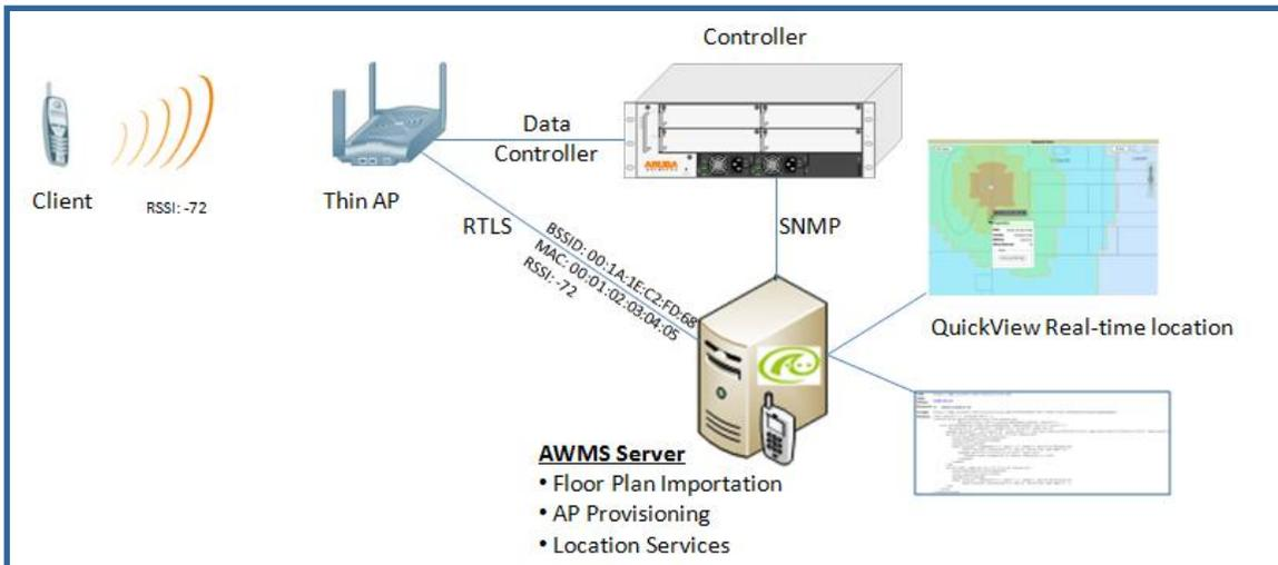
**Figure 27** Typical Tag Deployment
